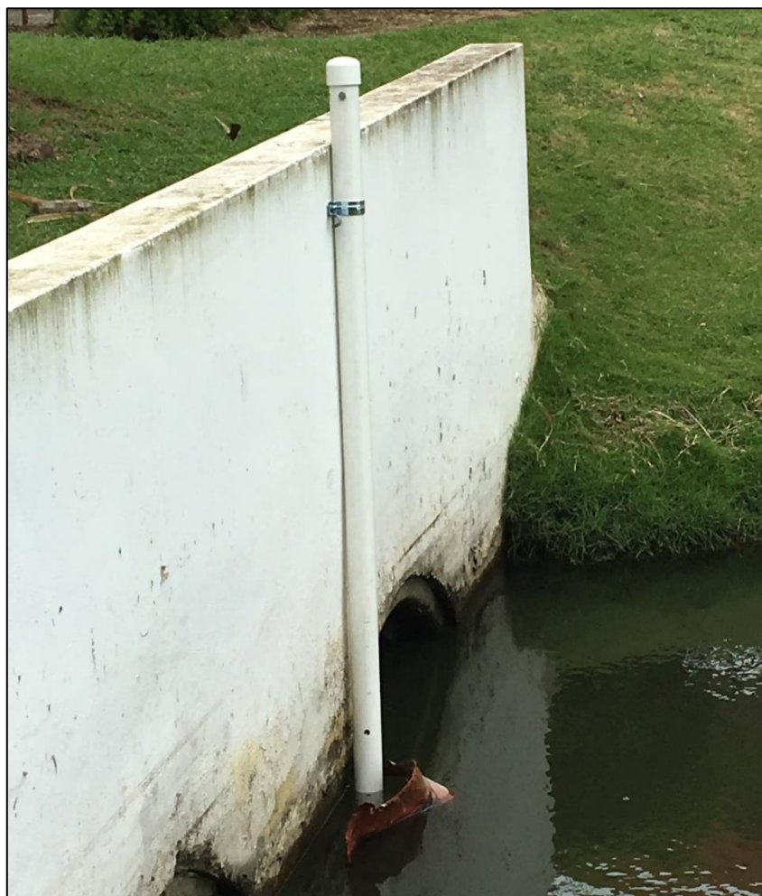
Photo 4 Installed level logger.
